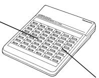
**16 Programmable Feature (PF) Buttons:** These buttons, once programmed, let you access various functions with one-touch operation.
