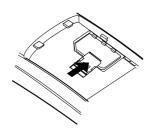
Place the battery onto the rear of the phone. Slide the battery up the body of the phone until it locks into place.
