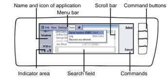
The communicator interface is turned on by opening the cover. The application that was active the last time the communicator was used is shown on the display.
