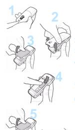
The SIM card is inserted under the telephone's battery. Ensure that the telephone is switched off and the charger disconnected.
