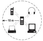
Every Bluetooth™ device has a unique address and a name. This is how the intended communication partners can be guaranteed to connect. The security concept is based on a password that both devices exchange when they connect for the first time. These "trustworthy" partners can be included in a list. The password prompt is not required for future connections. For settings, see page 93.
